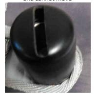
**NON CONFORM**: the plastic cap is worn, the safety pin may go out of its axis
