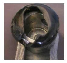
**NON CONFORM**: the cap has moved up on the sling, the safety pin may go out of its axis
