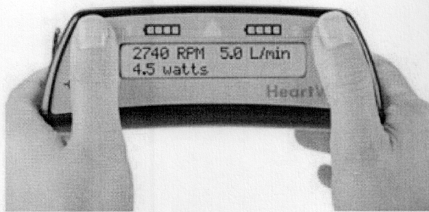
Figure: HeartWare Ventricular Assist Device Controller, a small computer that monitors the pump
