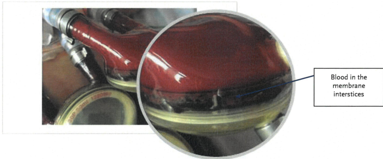
Figure 3: Identifying a defect of the blood-side layer: Blood in between the membrane layers in front of the stabilization ring.
